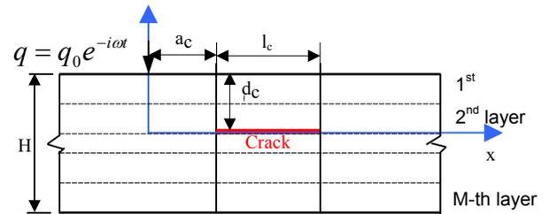
A M-layers anisotropic laminated plate with a horizontal crack
