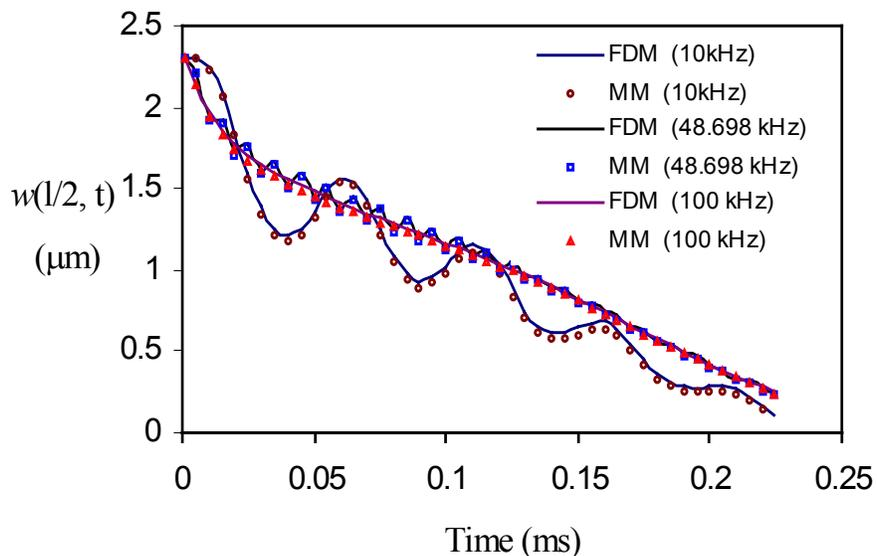
Figure 2. Simulation of pull-in dynamics for a set of sinusoidal input voltage with full model and macromodel
