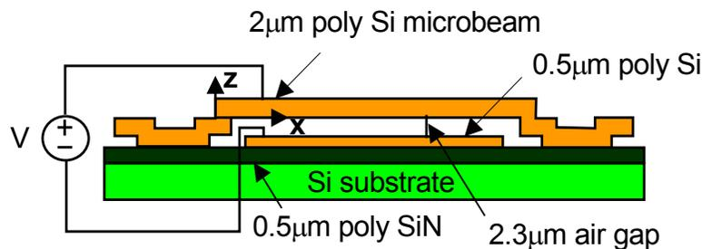
Figure 1. A MEMS device modeled as doubly-clamped beam
