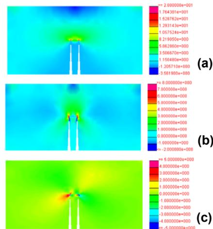
Fig. 3 Sample computation to test the relay model. The interference between two close cracks within a rectangular plate. (a)  $\sigma_{xx}$ ; (b)  $\sigma_{yy}$ ; and (c)  $\sigma_{xy}$ .
