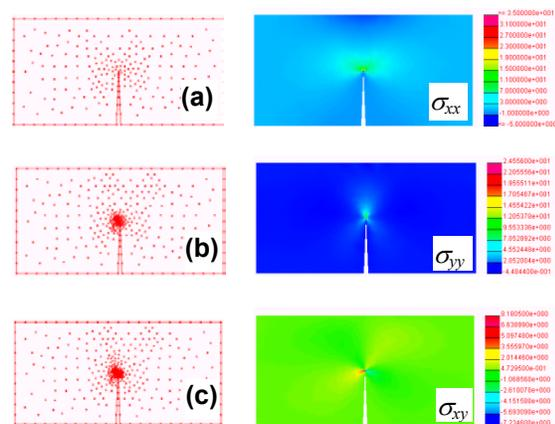
Fig. 5 A rectangular plate with a single crack. The refinement process and the final stress distributions.
