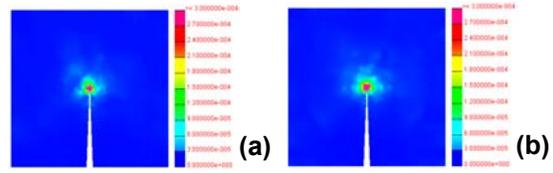
Fig. 3 Error distribution within a square plate containing a single crack. (a) estimated error; and (b) analytical error.
