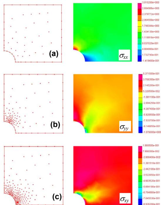
Fig. 4 A square plate with a hole. The refinement process and the final stress distributions.
