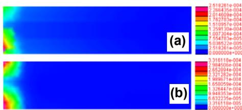
Fig. 1 Error distribution within a cantilever beam. (a) estimated error; and (b) analytical error.
