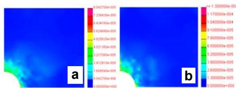
Fig. 2 Error distribution within a square plate with a hole at the centre. (a) estimated error; and (b) analytical error.
