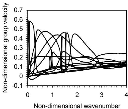
Fig. 1 Group velocity spectra for a composite cylinder.
