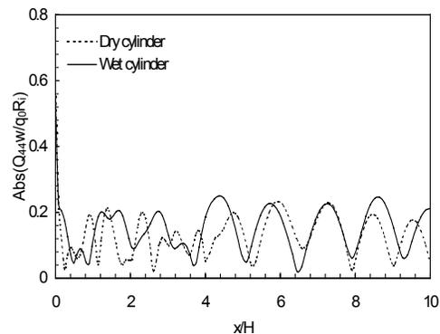
Fig. 3 Surface displacement of a fluid-loaded composite cylinder with an interior radial crack.
