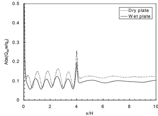
Fig. 2 Surface displacement of fluid-loaded composite plate with surface-breaking cracks.
