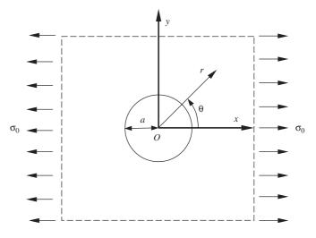
Fig. 9. Infinite plate with a circular hole subjected to unidirectional tension.
