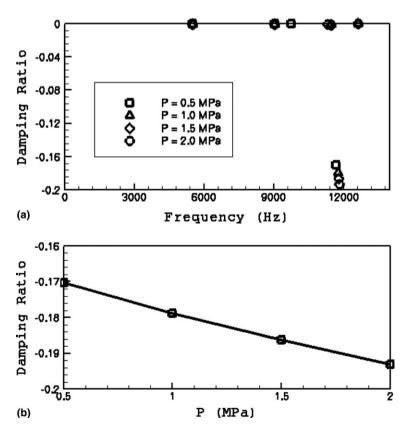
Fig. 4. (a) Variation of the damping ratio with frequency for different hydraulic pressures; (b) variation of the damping ratio with hydraulic pressure at frequency 12 kHz.
