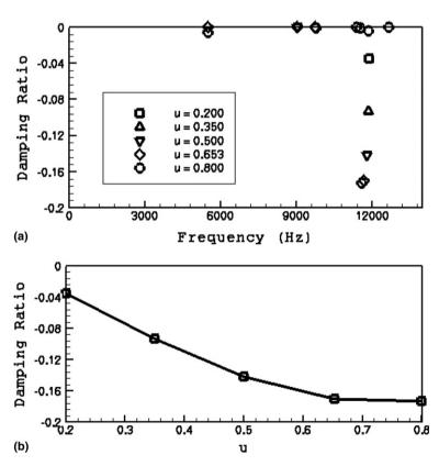
Fig. 3. (a) Variation of the damping ratio with frequency for different friction coefficients; (b) variation of the damping ratio with friction coefficient at frequency 12 kHz.
