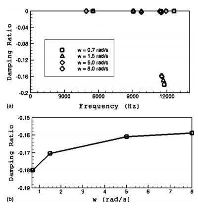
Fig. 5. (a) Variation of the damping ratio with frequency for different rotational velocities of the disc; (b) variation of the damping ratio with rotational velocity of the disc at frequency 12 kHz.
