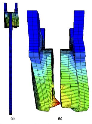
Fig. 9. Vibration mode of the disc brake system at frequency 12 kHz.
