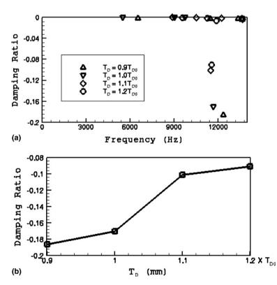
Fig. 7. (a) Variation of the damping ratio with frequency for different disc thicknesses; (b) variation of the damping ratio with thickness of the disc at frequency 12 kHz.
