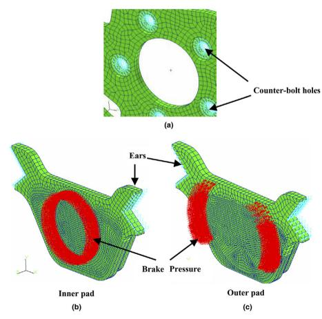
Fig. 2. Constraints and loadings of the disc brake system.
