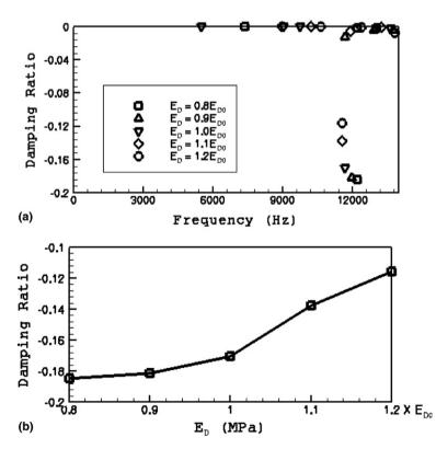
Fig. 6. (a) Variation of the damping ratio with frequency for different Young's moduli of the disc; (b) variation of the damping ratio with Young's moduli of the disc at frequency 12 kHz.
