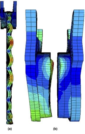
Fig. 10. Vibration mode of the disc brake system at frequency 9766 Hz.
