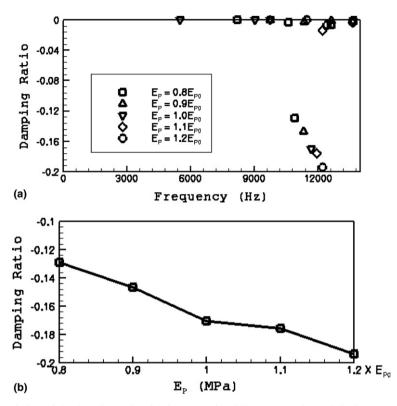
Fig. 8. (a) Variation of the damping ratio with frequency for different Young's moduli of the back plates of the pads; (b) variation of the damping ratio with Young's moduli of the back plates of the pads at frequency 12 kHz.
