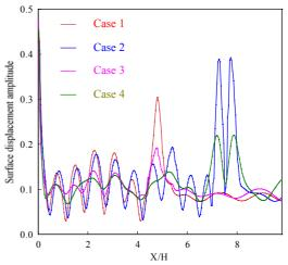
Surface displacement amplitudes used as the input of neural networks
