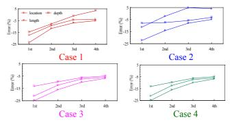
Errors of crack parameters detected by neural networks when no noise involved in the response data
