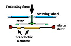
Fig.3. Schematic view of an elastic fin ultrasonic micromotor
