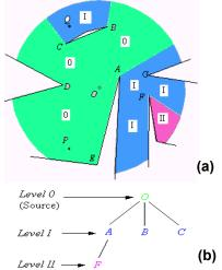
Fig. 1 A relay model constructed within an influence domain containing numerous irregular boundary fragments. (a) the relay regions; (b) the network of relay points.
