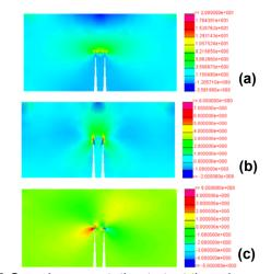
Fig. 3 Sample computation to test the relay model. The interference between two close cracks within a rectangular plate. (a)  $\sigma_{xx}$ ; (b)  $\sigma_{yy}$ ; and (c)  $\sigma_{xy}$ .
