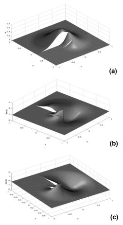
Fig. 2 Surface plots of the cubic spline weight function by the relay model. (a) w; (b)  $w_{,x}$ ; and (c)  $w_{,y}$ .
