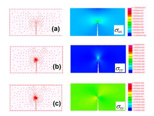
Fig. 5 A rectangular plate with a single crack. The refinement process and the final stress distributions.
