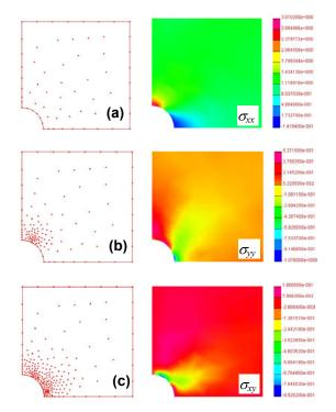
Fig. 4 A square plate with a hole. The refinement process and the final stress distributions.
