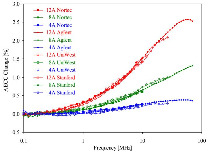
Figure 2 AECC change measured by four different instruments on three IN718 specimens of different peening intensities.
