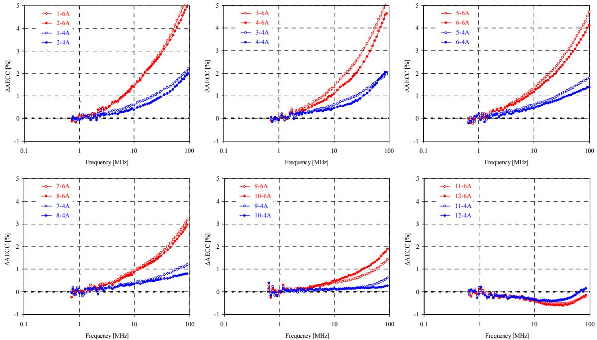
Figure 8 Apparent eddy current conductivity change in the twelve shot-peened IN718 specimens listed in Table 1.
