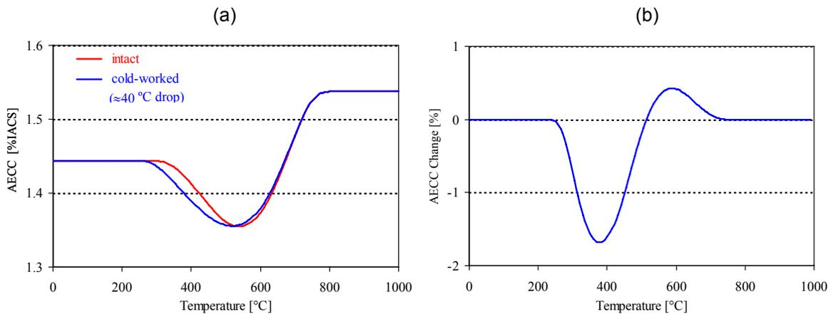
Figure 6 A schematic illustration of how the presence of cold work reduces the transition temperature at which thermally-activated microstructural evolution takes place in the material (a) and the resulting AECC change between the cold-worked surface and the intact interior (b).
