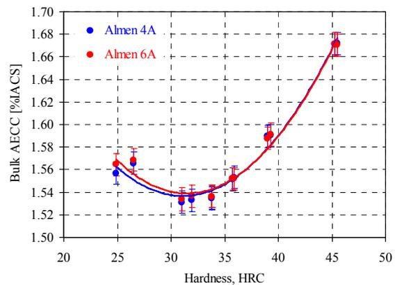
Figure 7 Bulk AECC versus Rockwell C hardness in twelve shot-peened IN718 specimens of Almen 4A and 6A intensity.
