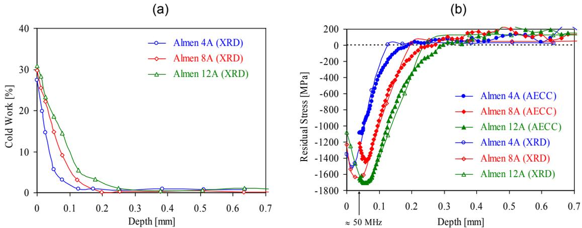
Figure 4 XRD profiling of near-surface cold work (a) and residual stress (b) profiles compared to the inverted eddy current residual stress profile in shot peened IN100 specimens of Almen 4A, 8A and 12A peening intensity levels.
