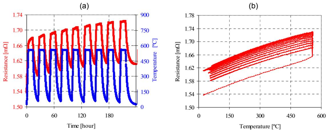
Figure 5 Variation of temperature and electric resistance in IN718 at 550°C peak temperature.
