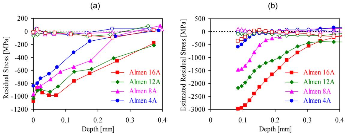
Figure 3 Comparison of destructive XRD residual stress profiles (a) and the estimated residual stress profiles (b) calculated from the measured AECC change for as-forged Waspaloy specimens of four different peening intensities (solid symbols represent as-peened specimens and empty symbols represent fully relaxed specimens after 24-hour heat treatment at 900 °C).
